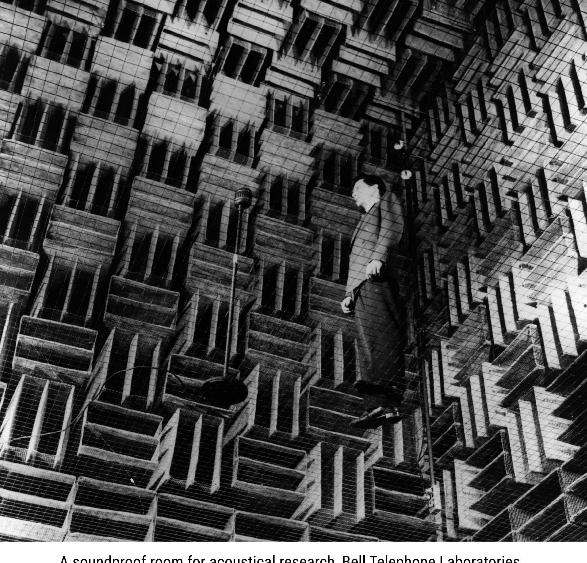
A soundproof room for acoustical research, Bell Telephone Laboratories. Photo by Keystone/Hulton Archive. Via Getty Images.
